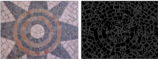
Fig. 10 – Exemplification of edge detection using Canny detector
